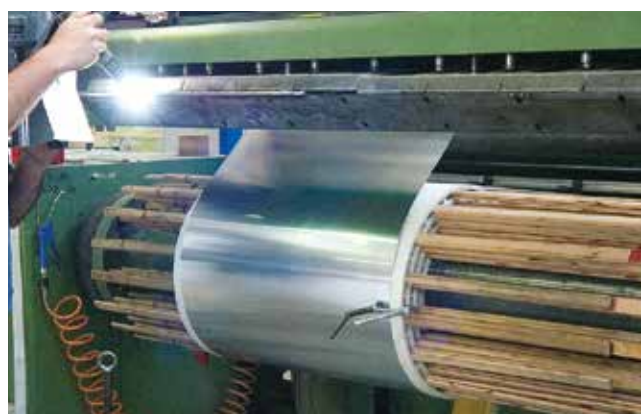
TIG welding in controlled atmosphere for LV connections.
