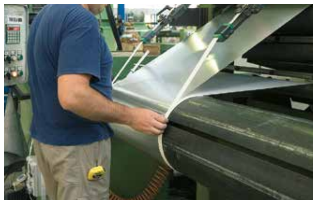
LV winding system
