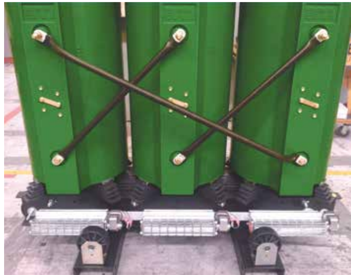
Example of transformer with ventilation bars
